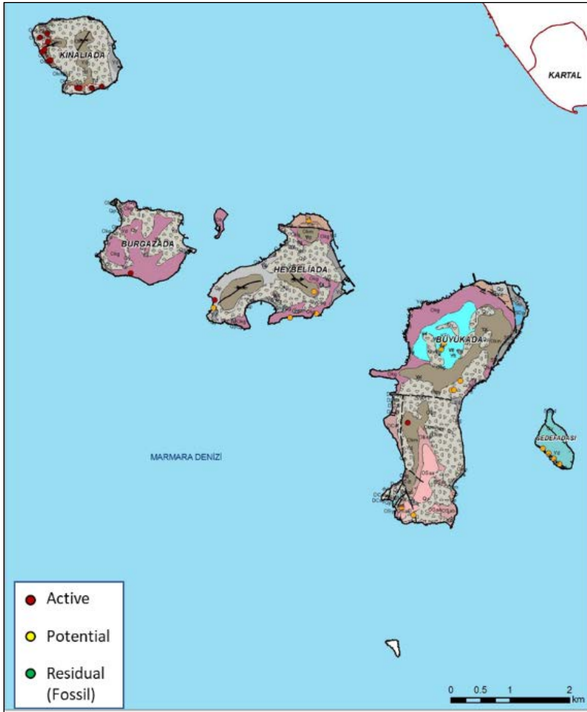
Figure 14. Mass Movement Locations of Adalar region according to activity status on the geology map (IMM, 2020).
