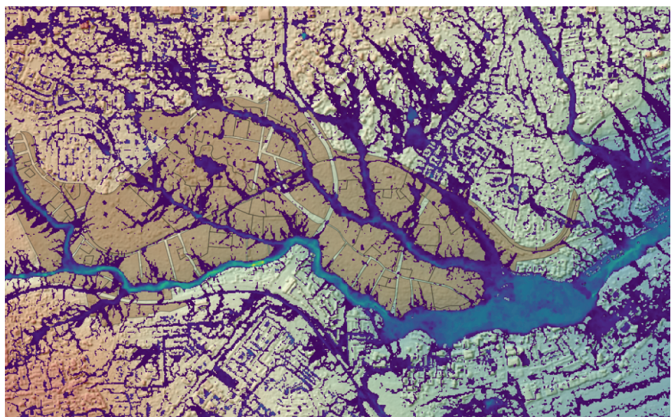
Flood event simulations that will later feed the calculation of impacts within each urban scenario.
